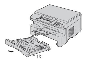
Before loading a stack of paper, fan the paper to prevent paper jams.
